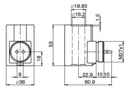
Coil with connection AMP Superseal / Metri Pack 150, 2-pole
